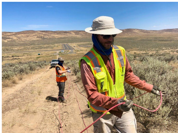
Army contractors Nick Pilar (front) and Cameron Stewart string wire along YTC Mettie Airstrip to conduct electrical resistivity surveys.
