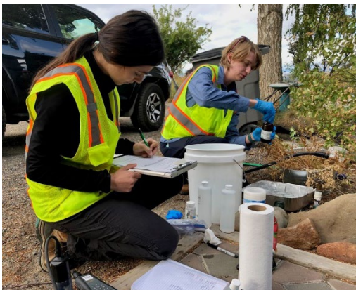
Army contractors Sarah Zurkee (left) and Michelle Schwartz, of Tanaq Environmental LLC, collect water samples to determine general chemistry that is used to design Point of Entry Treatment (POET) systems.
