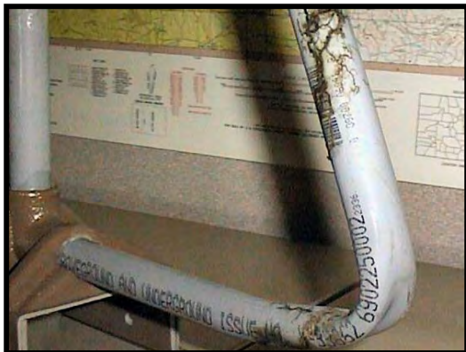
Figure 8-104. Flash marks on discourager.
