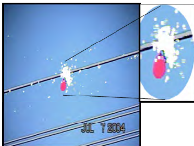
Figure 10-18. UV corona discharge from a flapper device mounted on an energized 345kV transmission conductor.
