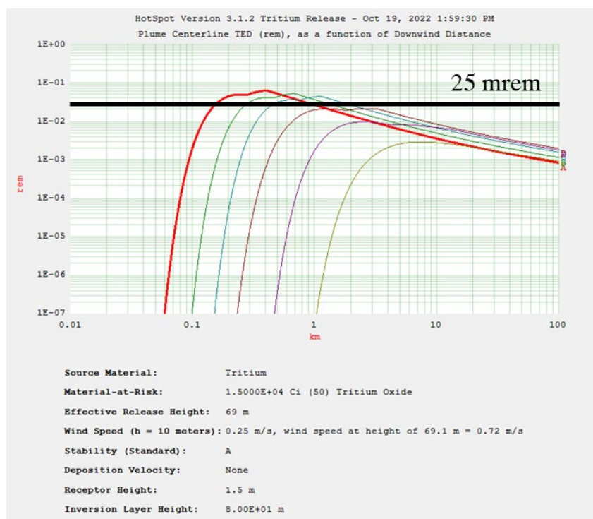
Figure 4. Graph of HotSpot Tritium Dispersal (Bold Red trace): Stability Class “A”, Stack Height = 16 m, Flow Rate = 2700 CFM, velocity = 15 m/s. Plots for classes B-F are inaccurate.
