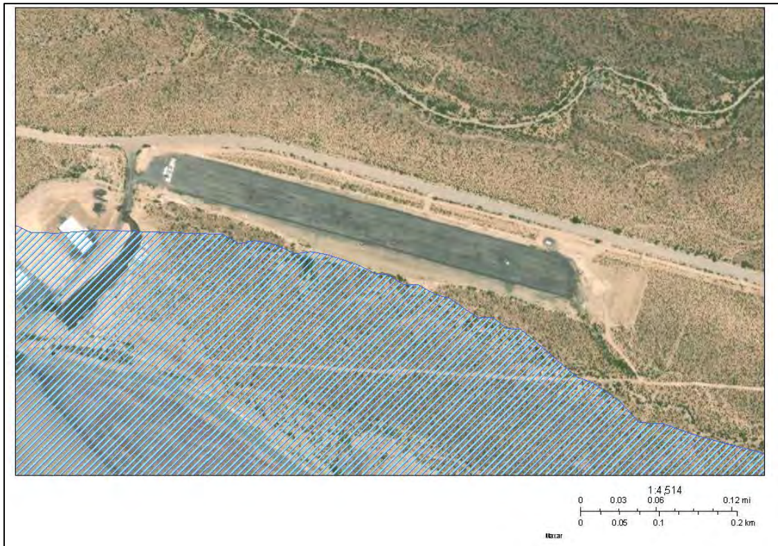
10 11 Figure 3-1. Special Flood Hazard Area (Zone A) Near ReDI Range
