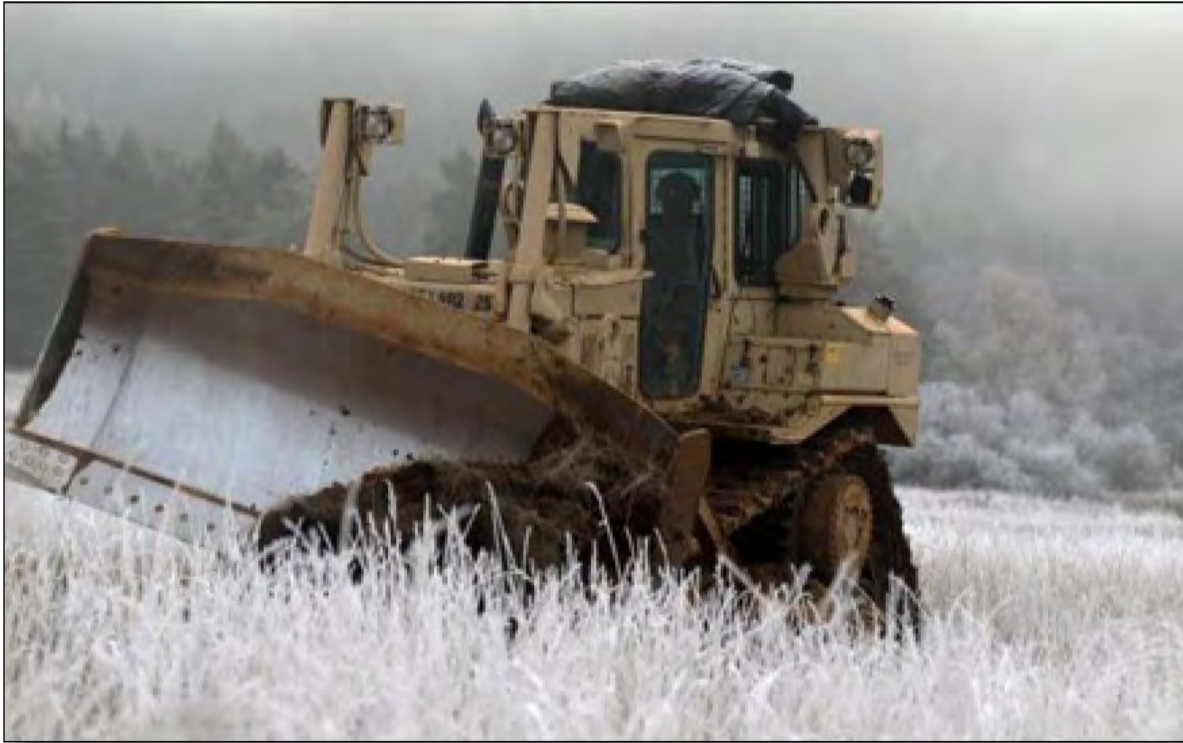
A D7 bulldozer is used to begin construction of a tank ditch.
