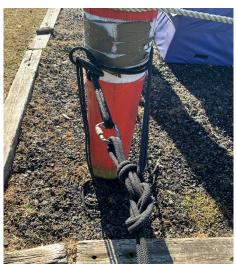
Wrap rope around anchor point, secure one, 51 KN steel locking carabineer, hook up rope and lock carabineer, wrap back around under first two strands and pinch against anchor point
