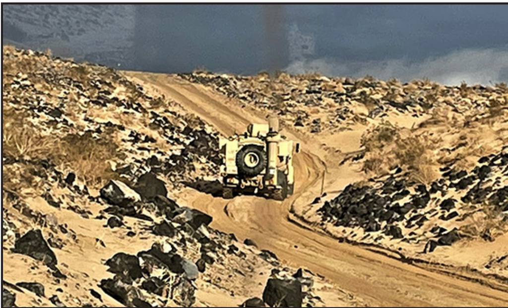
A mine-resistant, ambush-protected vehicle gets stuck while attempting to traverse a semi-improved trail at NTC.
