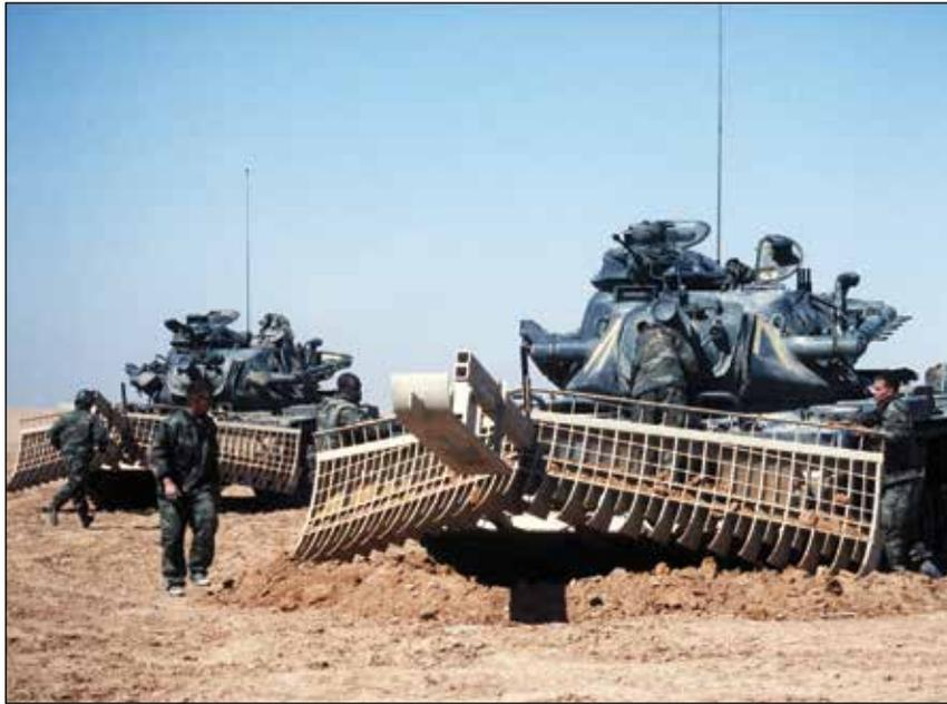
Figure 10.1. Members of the 72nd Engineer Company, 24th Infantry Division, test a mine-clearing rake attached to an M-728 Combat Engineer Vehicle (CEV) during Operation Desert Storm. Source: US Army Engineer School History Office Archives.
