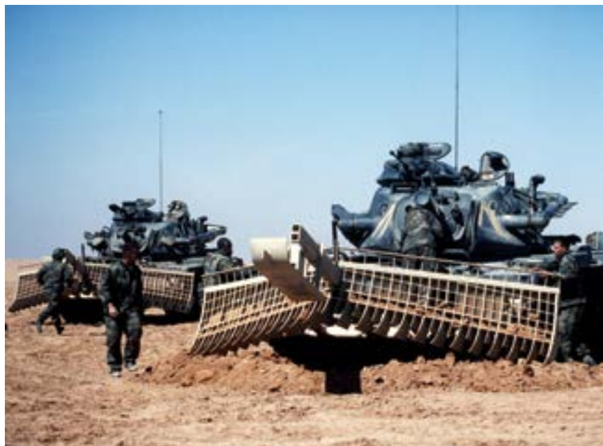
Figure 9.3. Members of the 72nd Engineering Company, 24th Infantry Division, test a mine-clearing rake attached to an M-728 Combat Engineer Vehicle. Photo courtesy of US Army Engineer School History Office.
