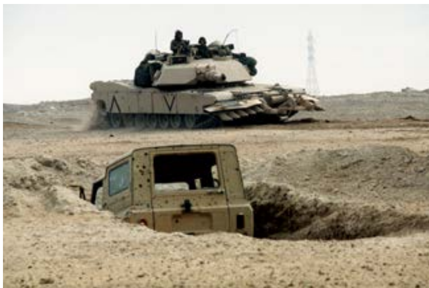
Figure 9.2. A Marine Corps M1A1 Abrams main battle tank equipped with a mine-clearing plow passes a truck in an abandoned Iraqi position. Photo courtesy of US Army Engineer School History Office.
