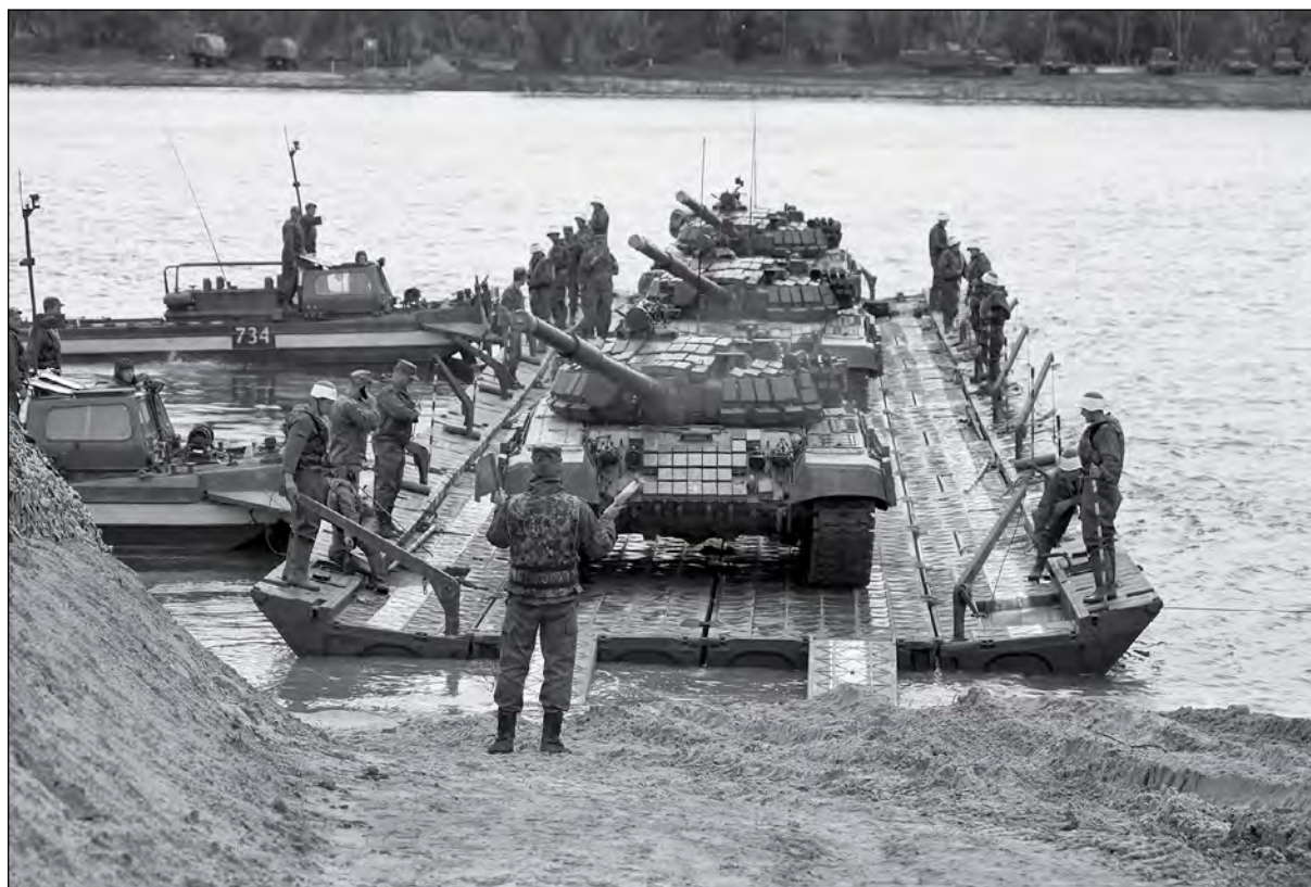
Pontoon bridge system functioning as a ferry
