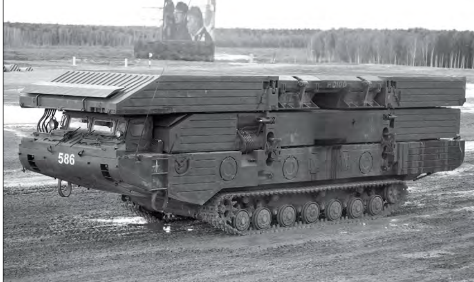
PMM-2M self-propelled ferry vehicle
