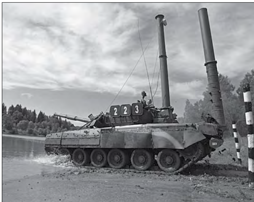
Tanks conducting snorkeling operations
