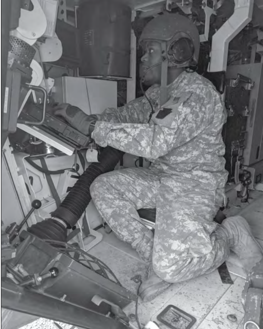
A truck commander occupies the surveyor's station and checks for onboard faults and alarms using the CBRN Detection Analysis Communication System.
