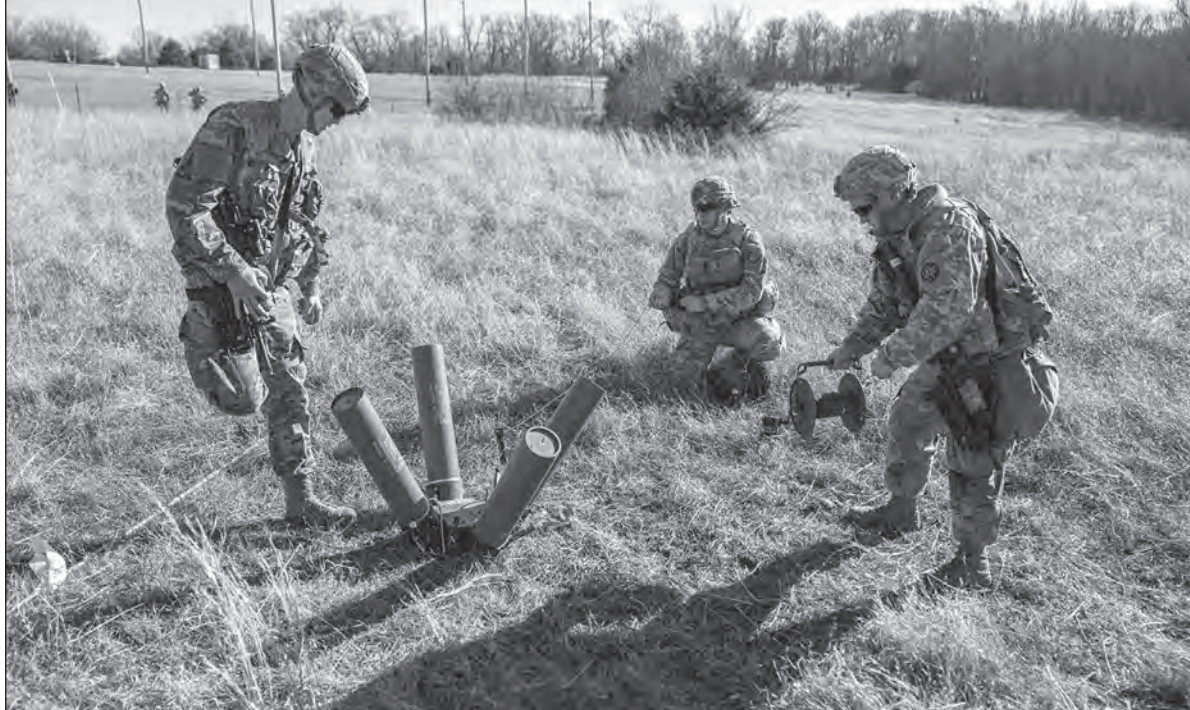
Soldiers install SAVO baseplate and Volcano canisters to form a SAVO pod.
