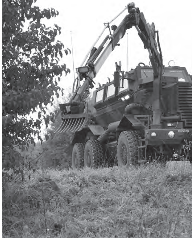
A U.S. Soldier uses the interrogation arm of a Buffalo mine-resistant, ambush-protected vehicle to examine a potential hazard.
