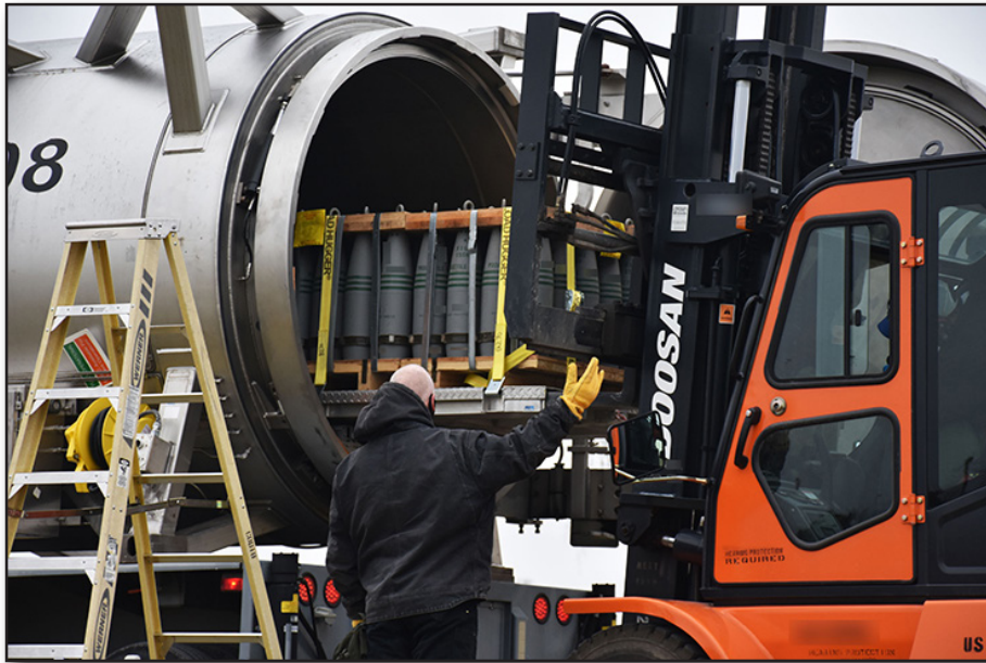
BGCA toxic materials handlers guide VX projectiles into an enhanced on-site container for demilitarization transfer.
