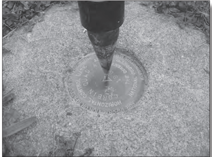
A typical survey monument is a brass cap set in concrete.
