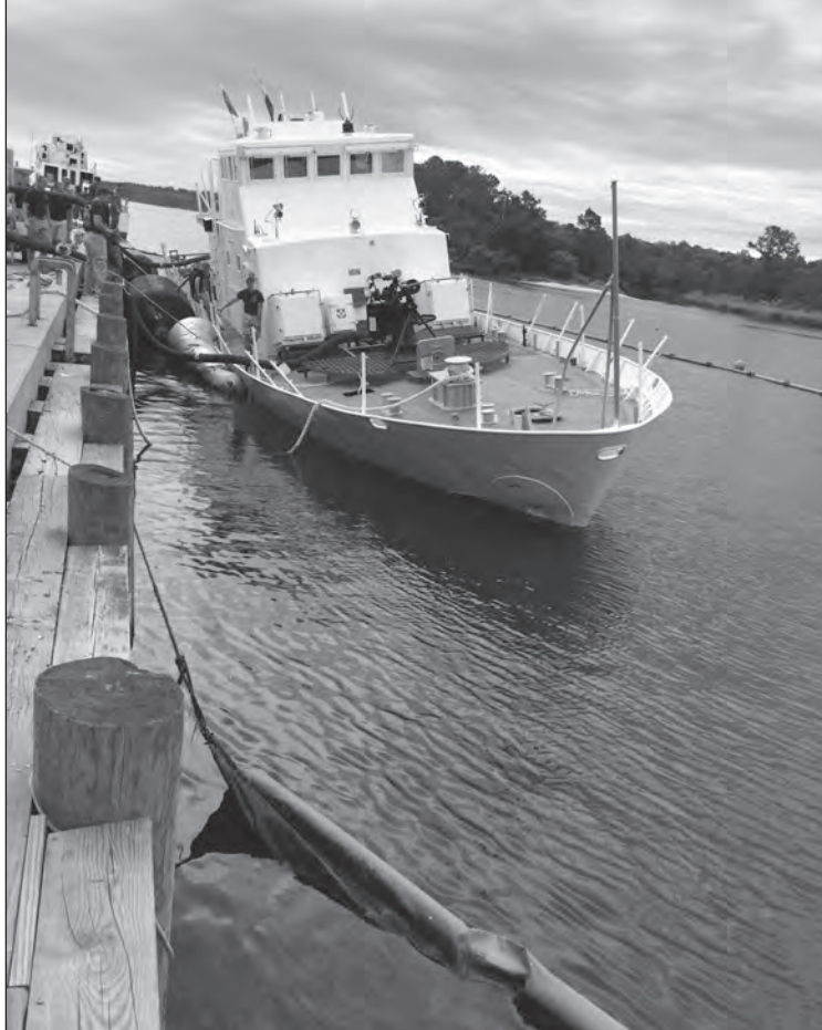
The vessel begins to list toward the pier during the intentional sinking phase.
