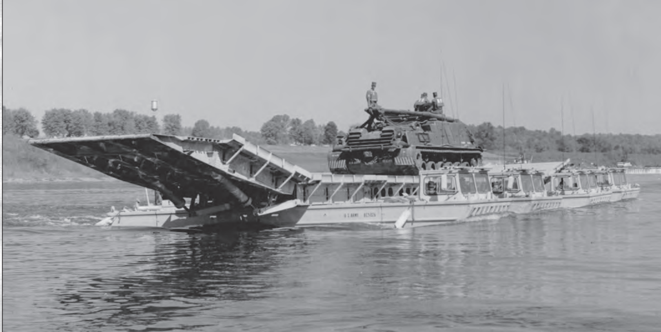
A four-float MAB raft on the Ohio River transports an M88 recovery vehicle.
