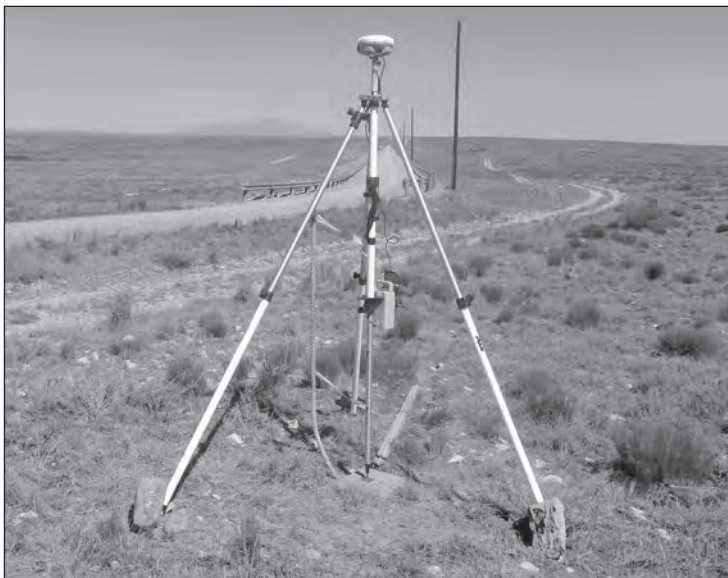
A high-accuracy global positioning system receiver is set up over a survey control monument.
