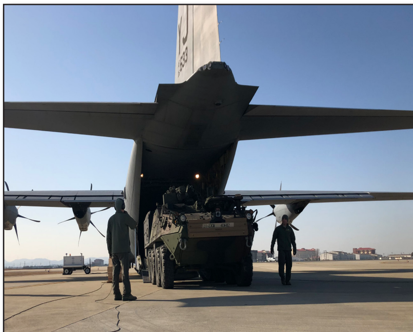
Crew members loading an NBCRV onto a C-130J Hercules aircraft
