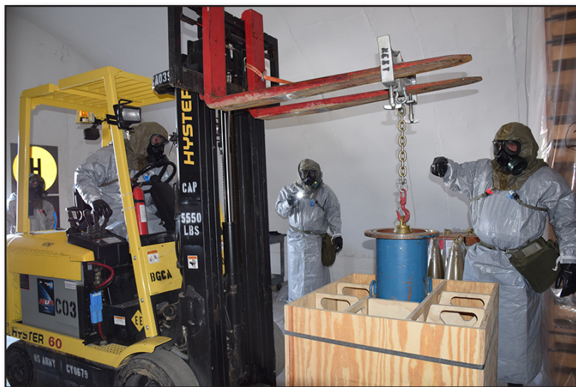
BGCA personnel demonstrate how to containerize a leaking chemical munition during an inspection.
