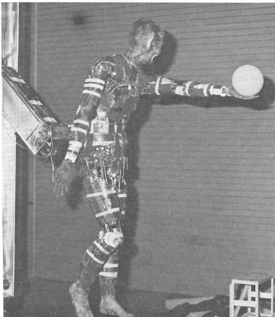
Manny is an anthropomorphic robot which will be used to test protective clothing.
