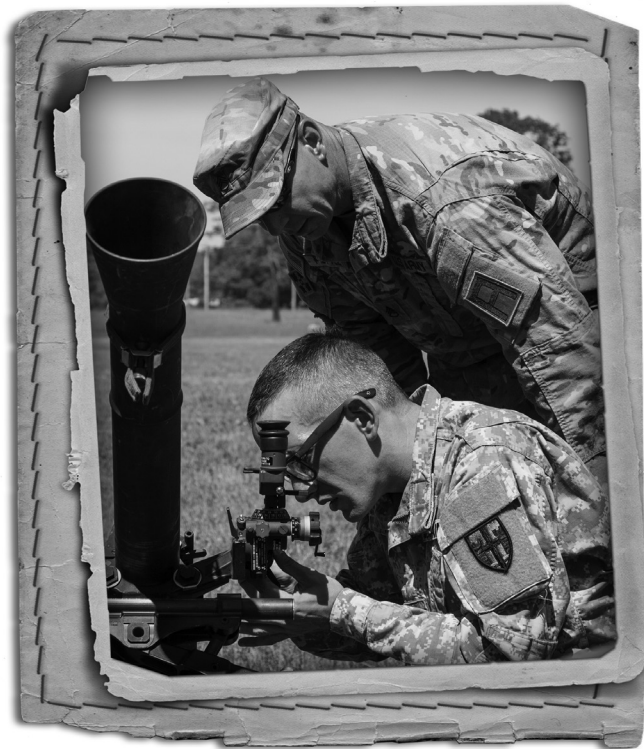
An OCT with the 157th Infantry Brigade teaches a mortarman with the 1st Battalion, 296th Infantry Regiment, Puerto Rican Army National Guard, how to adjust the aim on a mortar system. U.S. Army photograph by Sergeant Jarred Woods.
