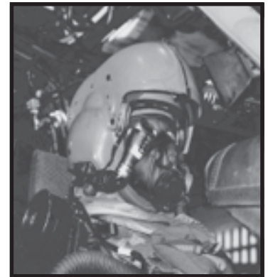
Mask interface with AH-64 Apache IHADSS
