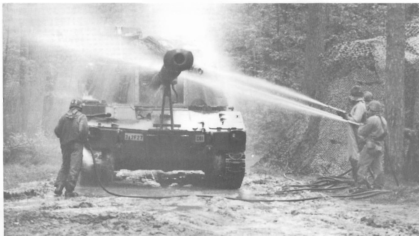
Above, an M109A2 self-propelled howitzer approaches a deliberate decon site. Below, the M109A2 undergoes decon.
