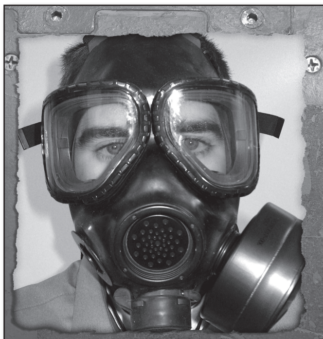
Oversized mask: The eyes fall below the center of the mask, and the hairline is under the periphery.
