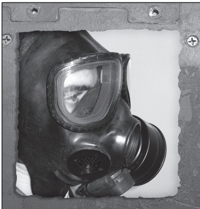
Oversized mask: The nose cup overlaps the eyes and field of vision.
