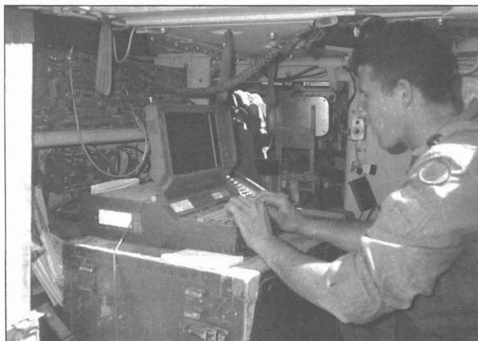
The Operations NCO of Company C, 317th Engineer Battalion, uses a situational awareness terminal of the Enhanced Position Location Reporting System (EPLRS) to track the company's movement.
