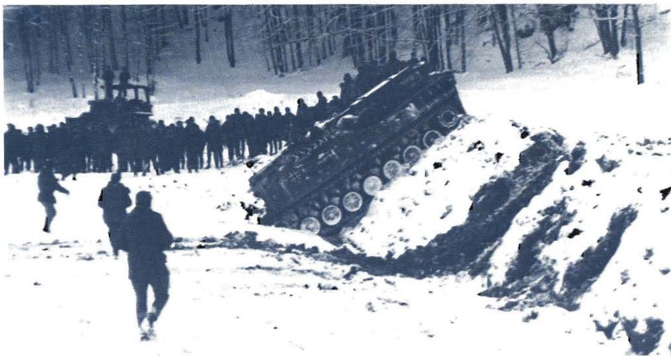
German recovery vehicle is stymied by an antitank ditch constructed by personnel of the 9th Engineer Battalion for a demonstration at the Hohenfels Training Area.
