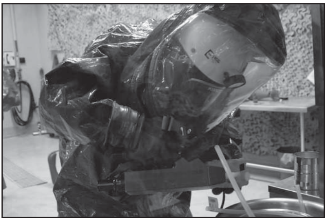
A member of the 93d CST employs an Improved Chemical-Agent Monitor and MultiRAE gas meter during site characterization of a clandestine laboratory in a lethal nerve agent environment at the CDTF.
