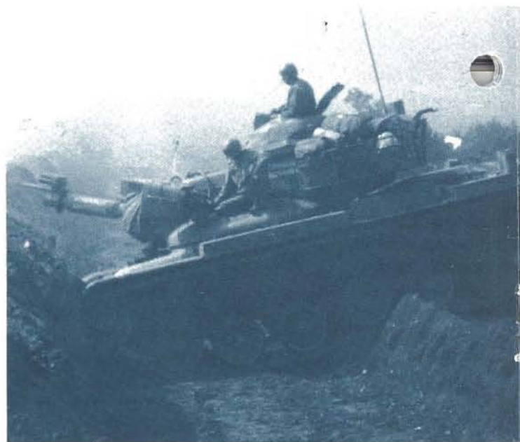
ATTACKING THE DITCH BY RAMMING. The gun is slewed. Ditch is too deep for enemy to turn it into a dug-in firing position.
