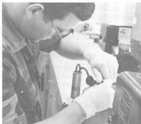
Top, SP4 Casey inserts batteries in AN/PDR27. Right, SP4 Casey prepares for a leak test of UDM-2.
