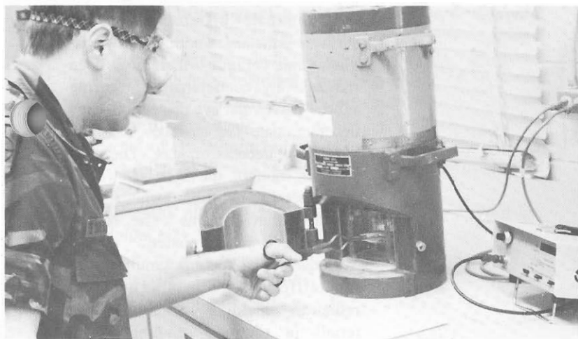
Left, 1LT Pool places smear into scaler to determine possible contamination. Above, a radiological laboratory practical exercise. Below, SSG Miller applies decontaminant to contaminated wood.
