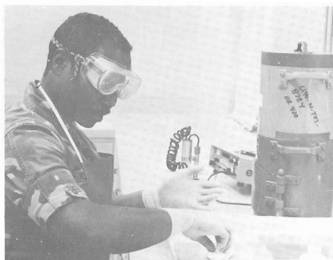
Left, 1LT Pool places smear into scaler to determine possible contamination. Above, a radiological laboratory practical exercise. Below, SSG Miller applies decontaminant to contaminated wood.
