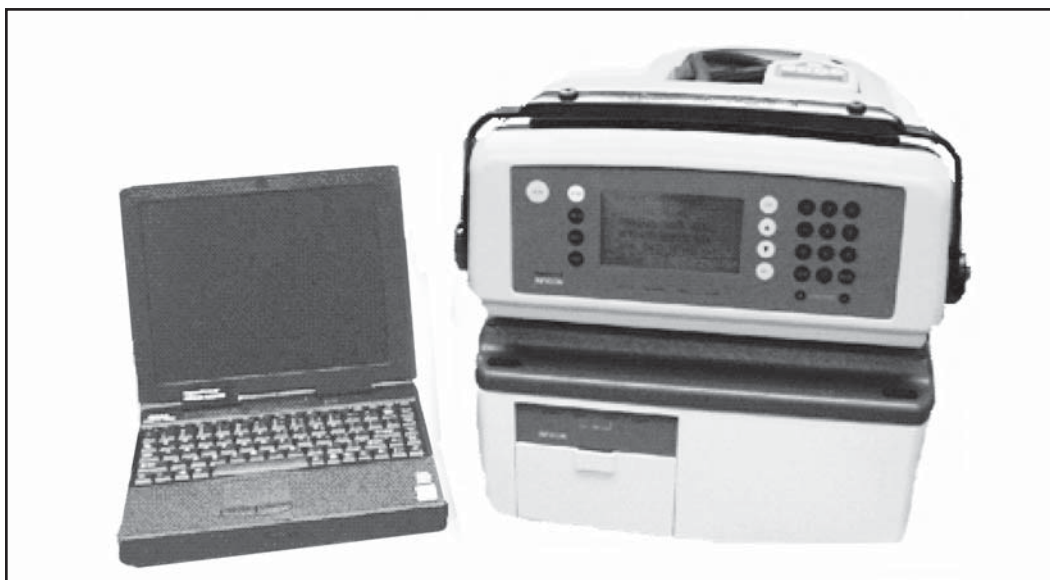
Figure 3. Gas chromatograph/mass spectrometer used to characterize suspected WMD agents or substances
