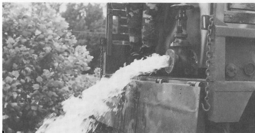
The four-inch gate valve (top left) easily fits the M12A1 adapter (top right). Over 1,600 gallons of water discharge in about ten minutes (above).
