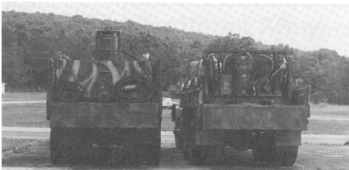
Bulk water tank (left) and tanked pump unit (right). A SANATOR has been loaded on top of the bulk water tank.
