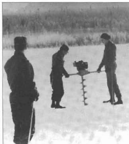
A profiling crew testing ice thickness.
