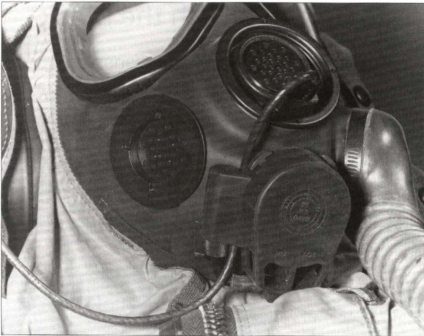
The proposed routing of the microphone cord in the M42 mask.
