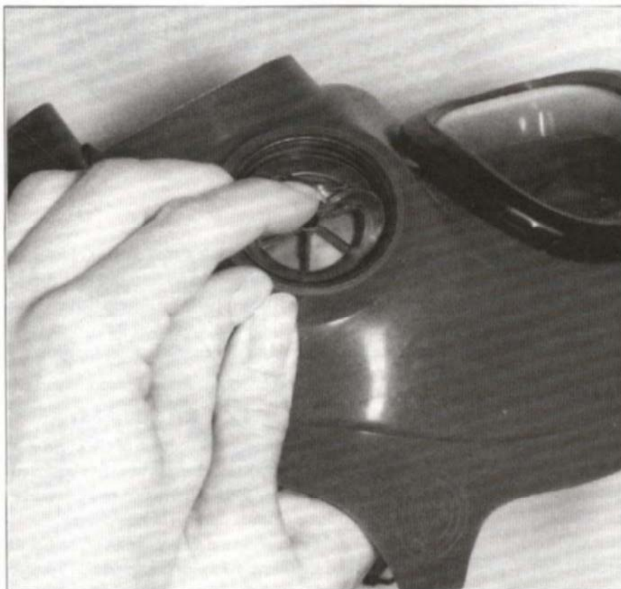
The proper attachment of the rubber inlet valve seat to the metal ring.
