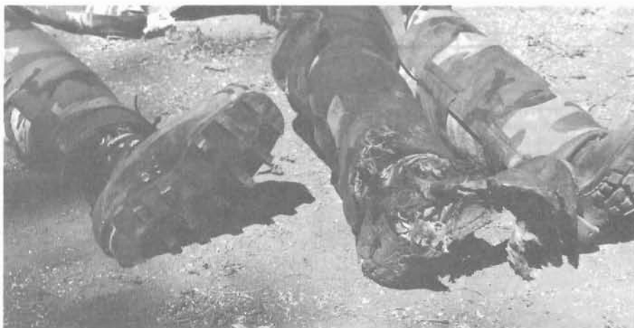
The protective boot on the left is intact after the blast that shredded its standard-issue neighbor.
