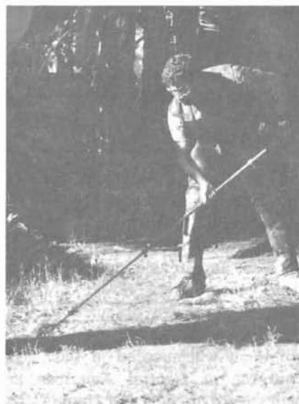
This simply-designed rake serves as a low-tech mine probe.
