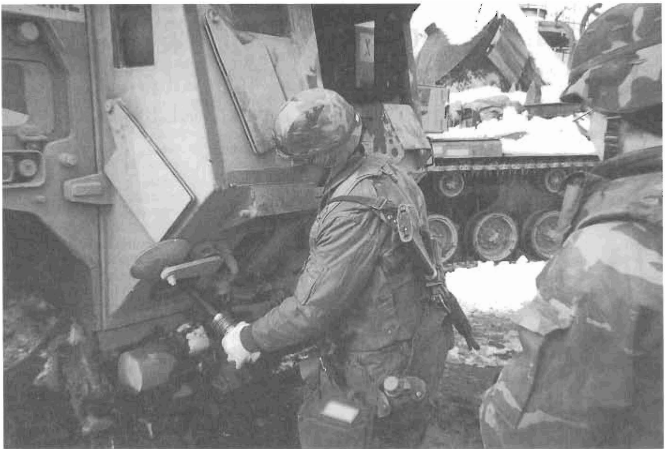
Reconnaissance squad leader using the mobile mass spectrometer to identify an environmental sample.
