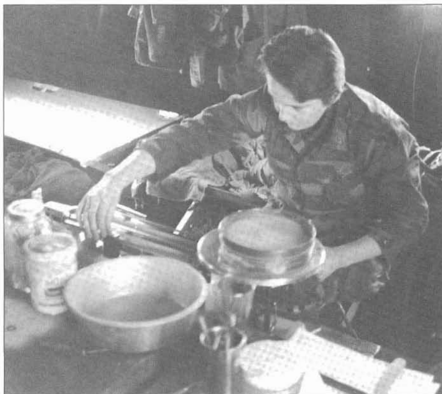
A materials specialist with the 802d Engineer Battalion in Korea weighs a soil sample for sieve analysis. On the spot soils testing makes engineers faster and more efficient in the field.
