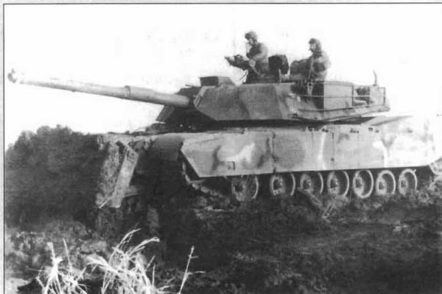
The crew of an M-1 tank uses a dozer blade being developed by the Army's Belvoir (VA) Research and Development Center to clear a path for the tank.
