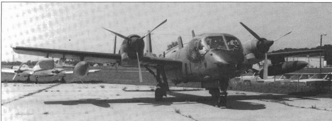
The OV-1D Mohawk was used to map the extent of flooding, locate seepage under levees, and survey the District for flood damage. (U.S. Army photo.)
