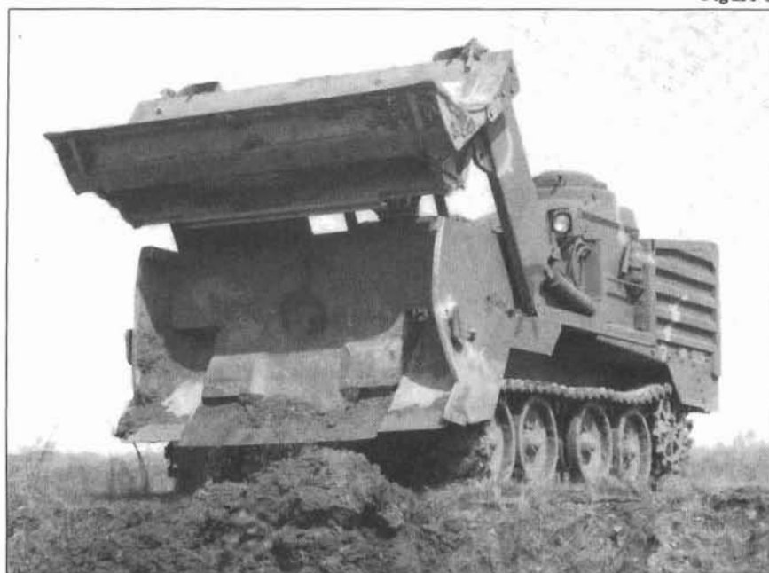
One of the ACE's many capabilities is dumping with its 2 1/2-cubic yard bucket. (U.S. Army photo.)
