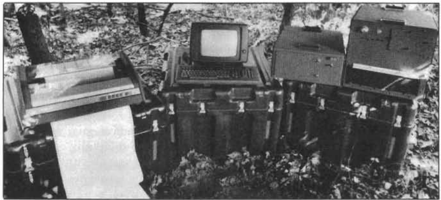
TACCS, an off-the-shelf computer and software system for battlefield combat service support missions. (Photo courtesy of Tactical Data Systems, General Electric.)
