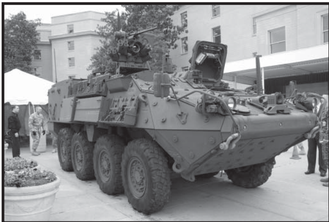
The Stryker NBCRV (displayed recently at the Pentagon) is an NBC testing lab on wheels.
