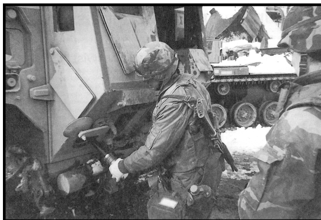
A reconnaissance squad leader uses the mobile mass spectrometer to identify an environmental sample.
