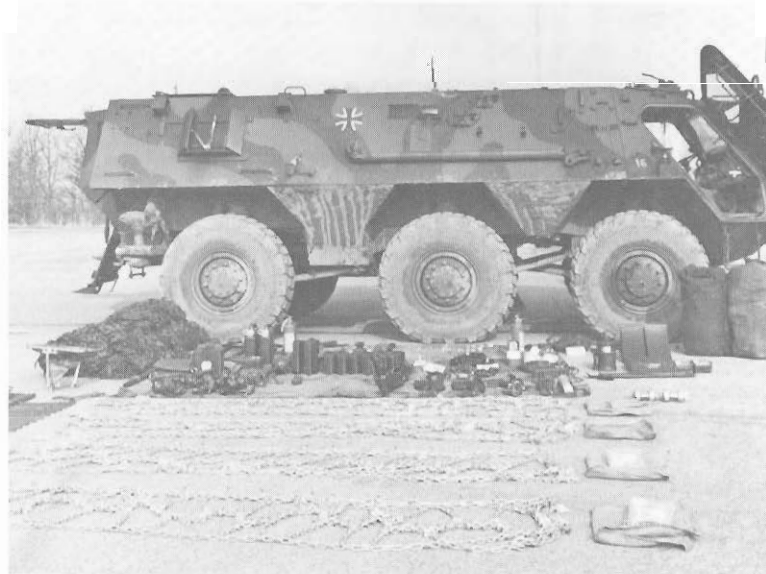
The TPz-1A3 NBC Reconnaissance System is shown below with basic issue items.
