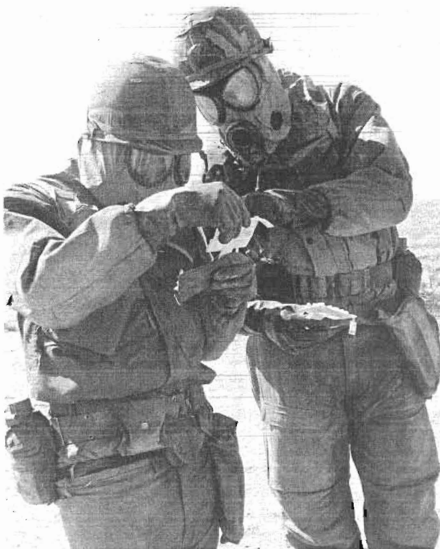
M256 TRAINS detector tickets are previously selected and marked to indicate nerve agent presence.
