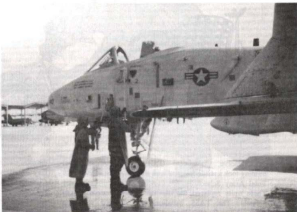
Above, Station 2. Two appliers (using long-handled mops with hot, soapy water) help remove gross liquid contamination. Because of the avionic equipment on the A-1, no DS2 was used. Below, Station 4. Sprayers rinse the aircraft using ordinary water.
