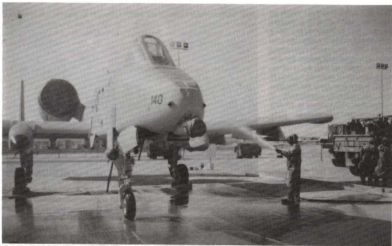
Station #1. Sprayer removes gross contamination using hot, soapy water.
