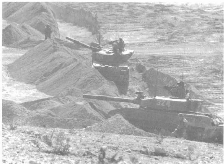
A poorly constructed antitank ditch is used by OPFOR armor as a fighting position. The tanks are M551s visually modified to resemble Soviet T72 tanks.
