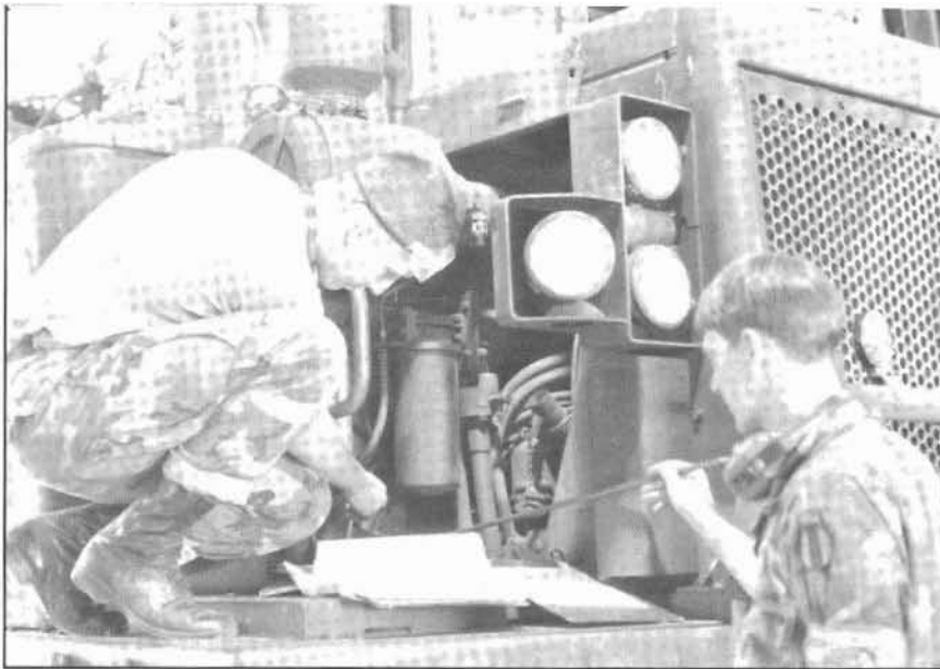
Trainees perform before-operation services on a 621B scraper, one of the newest pieces of equipment in the Army's system. The training for soldiers in the 62B10 MOS has been extended from over five weeks to nine weeks (photo by Ray Crosby).
