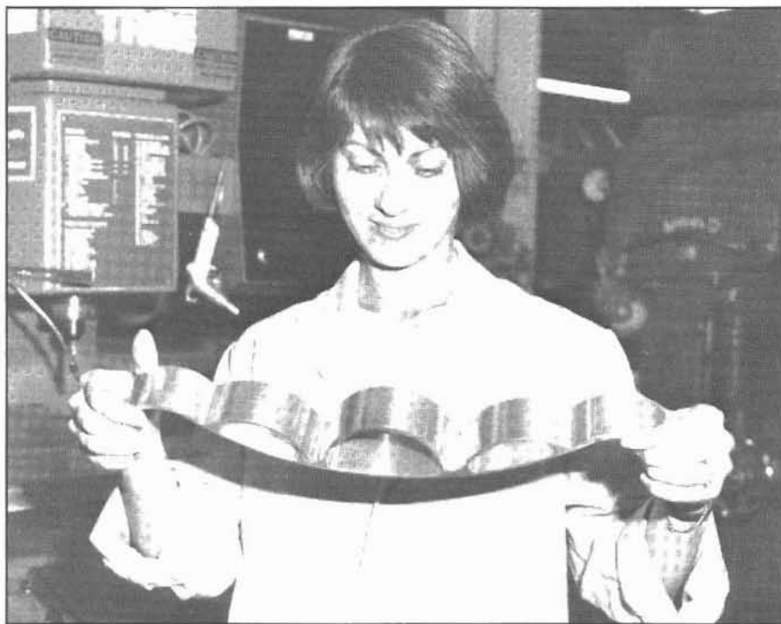
Catherine Kominos examines a completed model of her new bridge design. If tests are successful, this concept could reduce the weight of Army bridges by almost 20 percent (photo courtesy of Belvoir R&D Laboratories).
