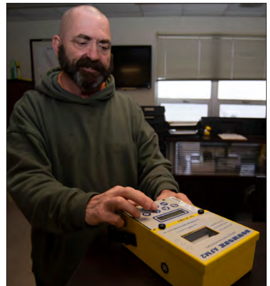
John Yohn, a flight operations specialist, prepares to use a decelerometer, which measures a vehicle's ability to brake on a given surface. The runway is checked in multiple places during inclement weather to ensure aircraft passenger safety.
