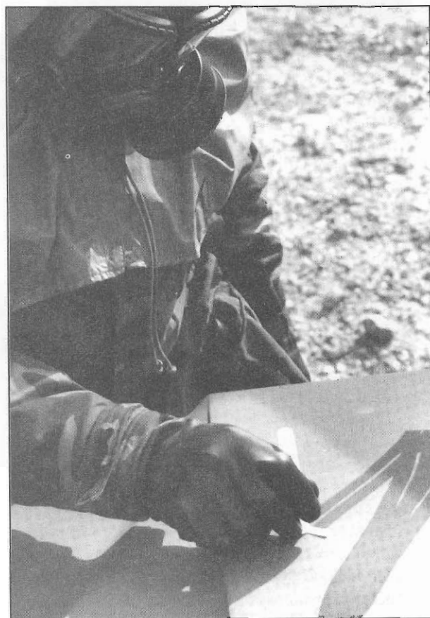
Soldier takes surface sample with the T-2 toxin kit from the XM294 chemical agent detector kit.
