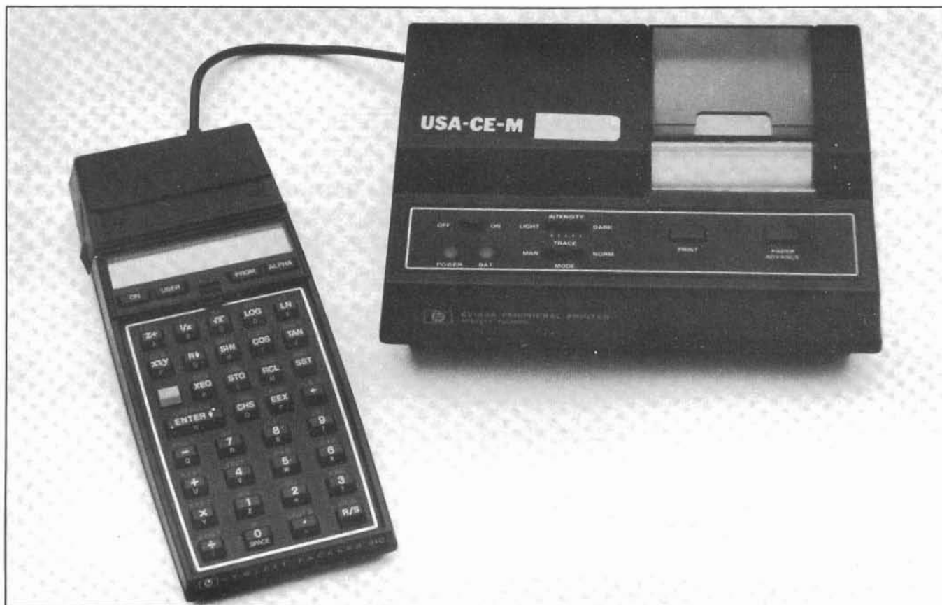
The HP-41c Engineer Programmable Calculator; plug-in, read-only-memory (not visible); card reader (inserted into top of calculator); and thermal printer.
