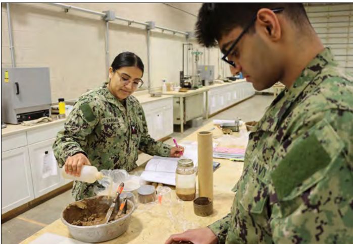
Navy Petty Officer 2nd Class Paula Vargas (left) and Navy Seaman Pratham Patel, CSFE students, test soil Feb. 15 to identify load-bearing capabilities.
