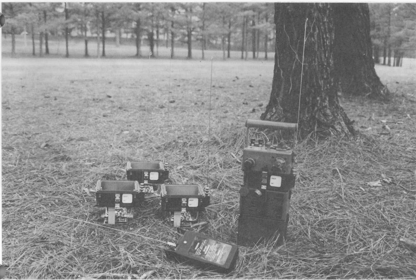
The kit components: one transmitter (front), four receivers (one mounted in the M43A1 detector). Note the thin whip antenna.
