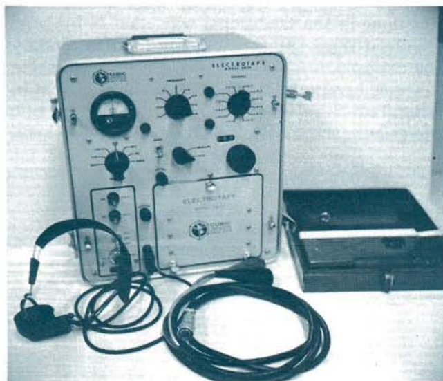
THE CUBIC DM20, A MICROWAVE DISTANCE MEASURING DEVICE (LEFT). A BATTERY DRIVEN PSYCHROMETER (WET & DRY AIR TEMPERATURE MEASURER) AND POCKET BAROMETER (RIGHT) ARE PART OF THE COMPLETE SYSTEM.
