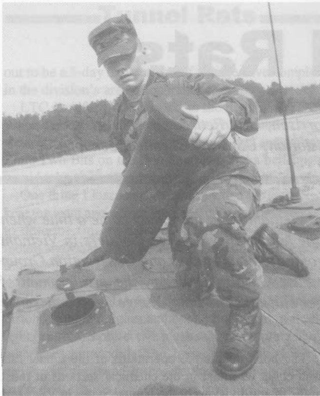
PFC Moss installs the detector air collector equipment on the biological integrated detection system.
