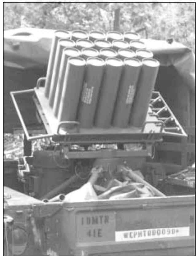
The Volcano (Light), scaled down to fit a HMMWV to match the mobility of a light fighter, creates a defensive minefield.
