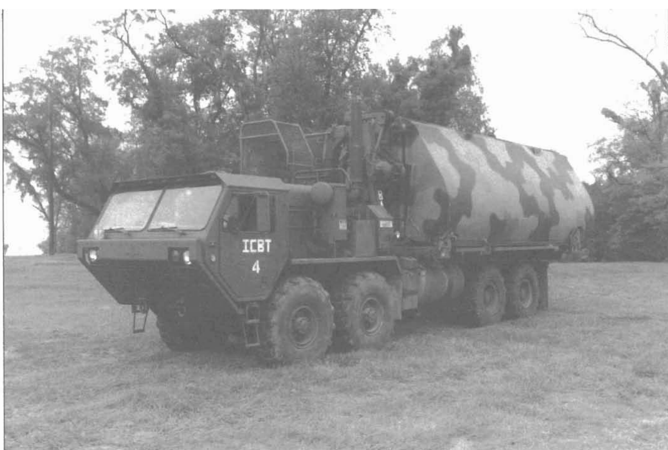
Common bridge transporter with improved ribbon bridge interior bay
